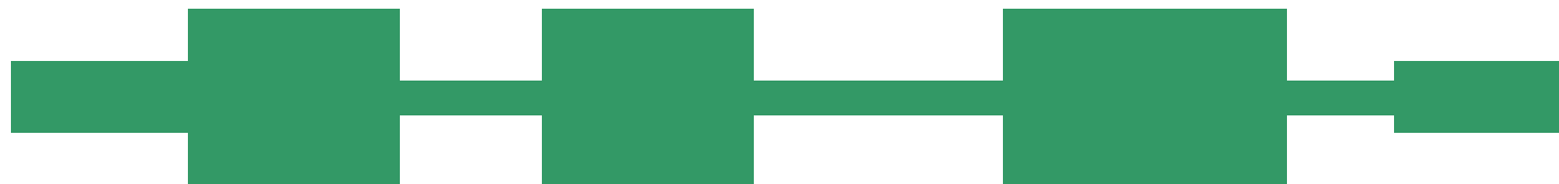
Microstripline Layout of Filter
